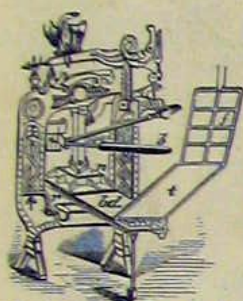
Columbian Printing press, 1038. t, tympan; f, frisket; r, rounce; b, bar; bd, bed; p, platen.
