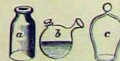
Receivers, p. 1095. a, cylindrical glass receiver; b, gas receiver; c, air-pump receiver.
