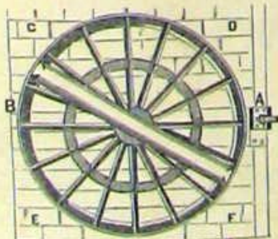
Mural Circle, p. 868. A, reading microscope; B C D E F, wall to which the circle is attached.
