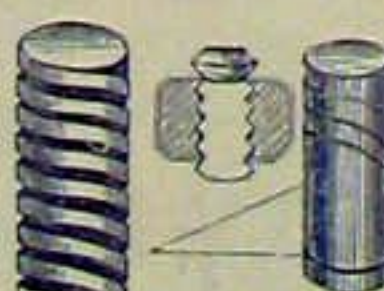
Screw, male and female, and thread, 1184.
